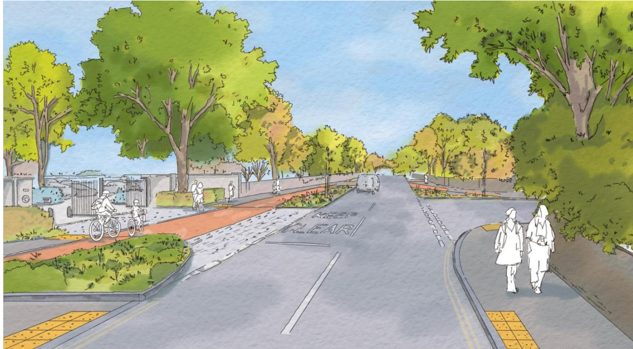
Shared cycle/pedestrian roadside facility ~£150k per 100m
