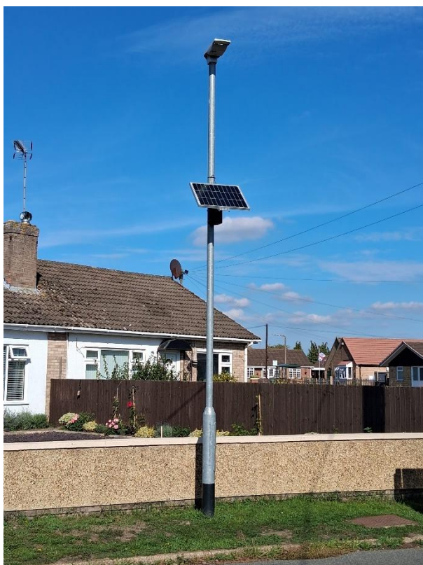
Figure 2-4 - Chapnall Road Zephyr indicative air quality monitor
