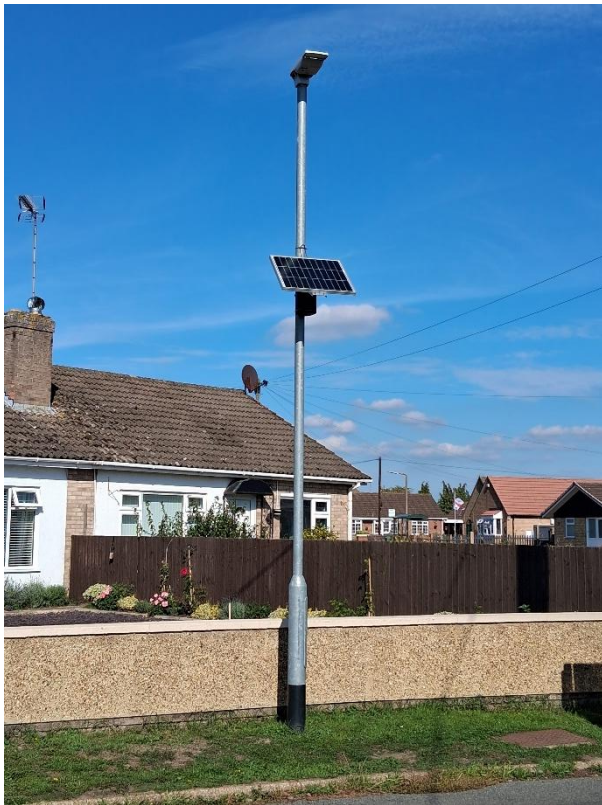
Figure 2-4 - Chapnall Road Zephyr indicative air quality monitor
